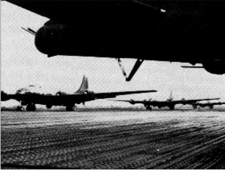
B-29s of the 98th Bombardment Group at Yokota are shown preparing to take off on a night mission in May 1953. The perforated steel planking shown here was used for temporary paving of hardstands.
